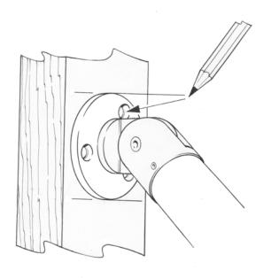
Pivot handrail bracket may vary to illustration - now with smaller flat edged back plate, with 4 fixings Create a pencil line and centred on the newel post position the handrail pivot bracket (supplied).
