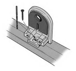
Fixing a string down the centre of the baseball can aid in ensuring clamps are set to the centre of the baserail
